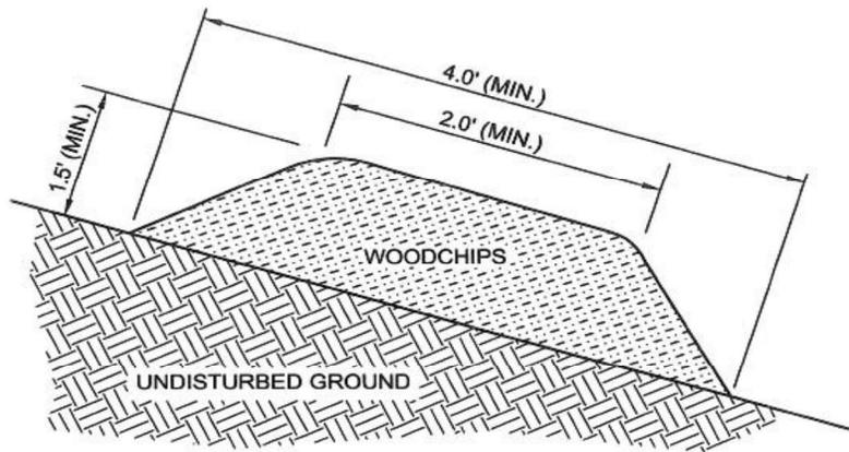
Prior to placement of the berm, obstructions such as tree limbs, large rocks, etc. shall be removed.
