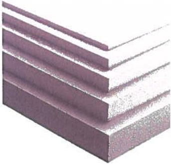
EXPANDED POLYSTYRENE FOAM (EPS) (Similar to the foam used for packing “peanuts”) R=3.6 to 4.0 per inch of thickness
